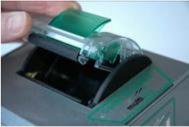
**Release the paper compartment cover using the green lever.**
