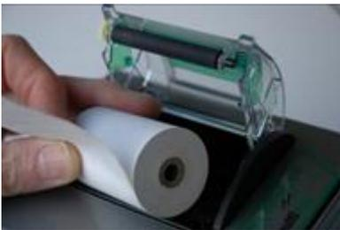
**Insert the thermal paper roll, noting paper orientation.**
